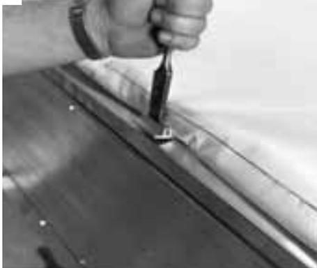
ABC provides the Tensioning Tool, or you can make your own from a blunted 1-1/2" wood chisel. The leverage provided by the tool makes it easy to hold the lever of the Tensioner flat against the frame, and easy to slide the Keeper in place.
