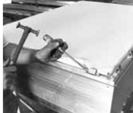
It may be necessary to release the corner Tensioners, adjust the position of the Tensioners over the Dowels, (inwardly to tighten, outwardly to loosen), to remove any remaining wrinkles in the corners.
