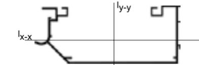
The neutral axes for the **Small A/Flexframe** are shown above.
