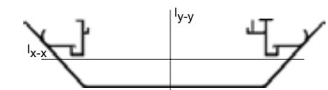
The neutral axes for the **Large A/Bleedframe** are shown above.
