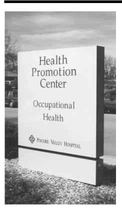
The 10" wide **Type I Conventional Frame** is the second largest frame system of this type. Internal service access is gained by removing one or more retainers and sliding the face left and right.
