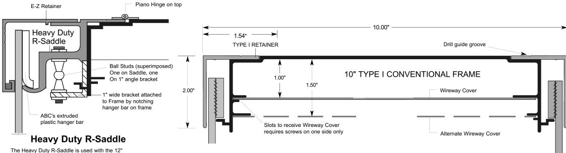
Conventional Frame for hinged faces, extending the width of the assembly to 15-1/2" wide. It provides space to mount the Ball Studs for attaching ABC's Gas Cylinder struts, which automatically opens the face and holds it open for hands-free internal service work.
