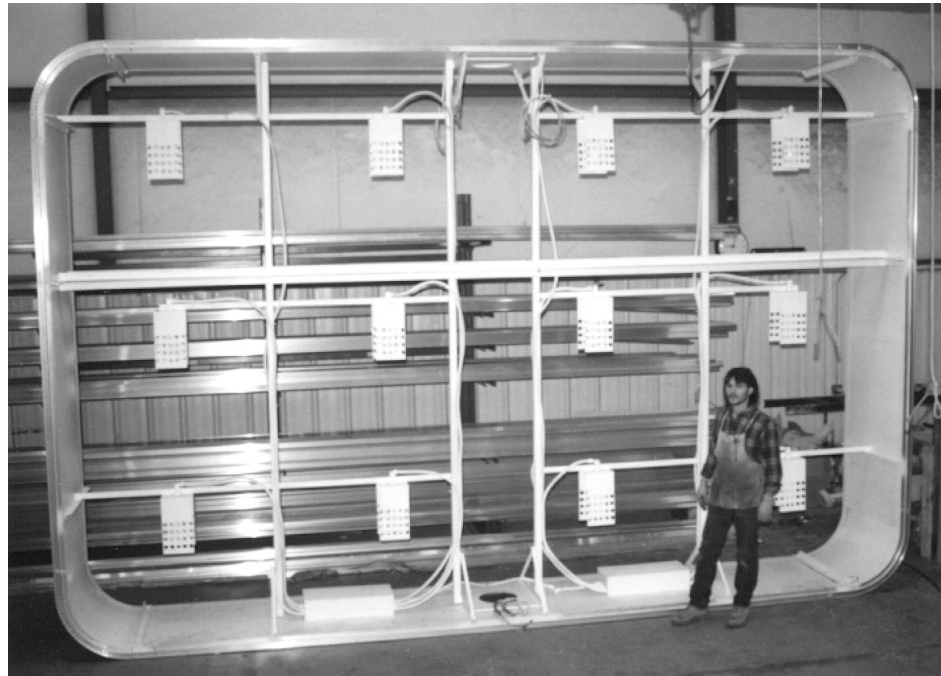
A 13' X 24' X 3' deep single-pole mount sign & metal halide lighting.
