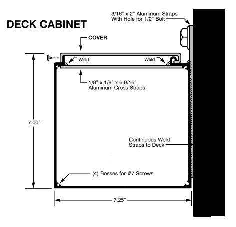
Their purpose is to hold the wide open mouth to its precise shape. Otherwise, when the Cover is opened for service, the heavy, cantilevered weight of the transformers and letters could spread the mouth, making it difficult to replace the screws in the Cover.
