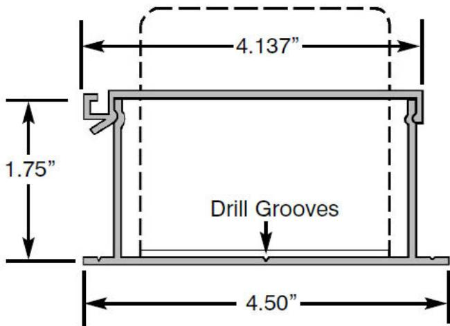
Our Small Ballast Wireway has been revised to make it taller and wider than it was originally, to give more room for wiring around the ballast. Note the new dimensions and features illustrated.
